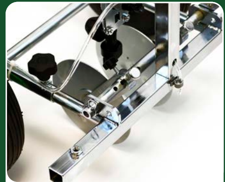
Easily-adjustable 50mm to 150mm (approx. 2" to 6") line width.
