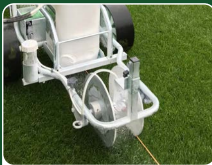
Unique front wheel gives the machine great precision & manoeuvrability for lifting over lines.
